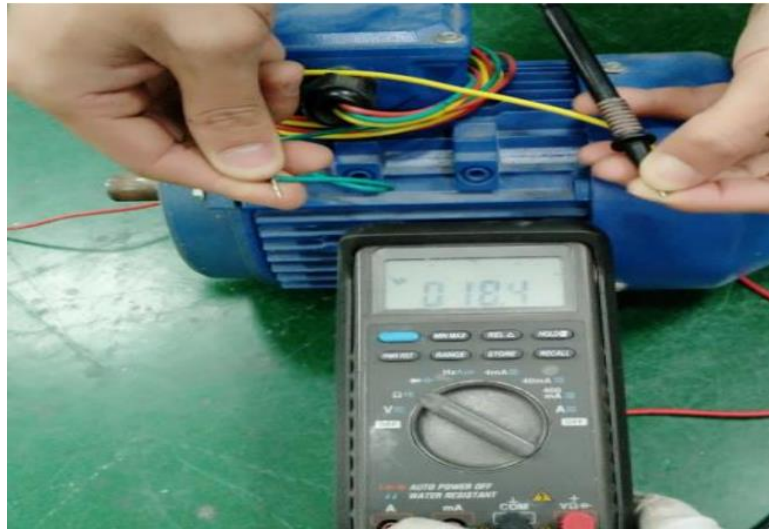
Figure. 12 Check if the winding is Open Circuit
