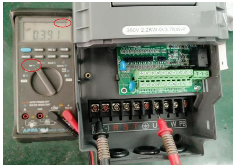
Figure. 3 Schematic Diagram of Three-Phase Upper Bridge Measurement in the Inverter Section
