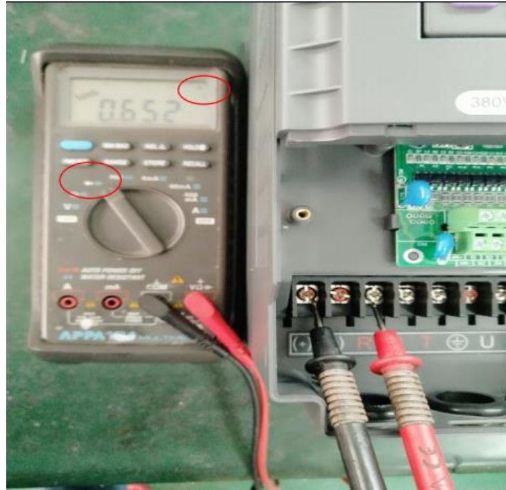
Figure. 1 Schematic Diagram of Three-Phase Upper Bridge Measurement in Rectifier Section
