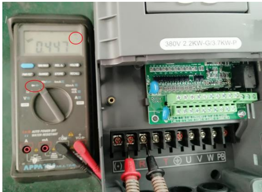
Figure. 2 Schematic Diagram of Three-Phase Lower Bridge Measurement in Rectifier Section
