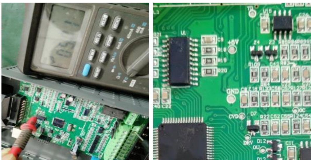
Figure. 9 Multimeter DC Gear, Black Pen on GND, Red Pen On +5V Up telegram E-01.E-03 or running telegram E-01.E-03
