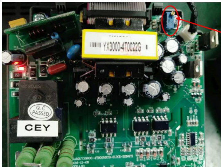
Figure. 11 Precise Adjustment can Calibrate the Bus Voltage of b-04
