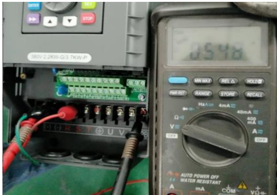
Figure . 5 Schematic Diagram of Braking Circuit Measurement
