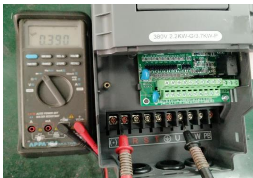
Figure. 4 Schematic diagram of Three-Phase Lower Bridge Measurement in the Inverter Section
