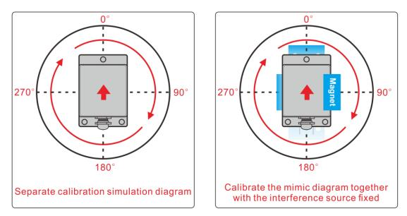
The starting point can be at any point of 360°, and it can rotate more than 1 circle on the spot Within 2 laps, the speed of rotation should be as uniform as possible, not too fast!
