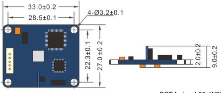
PCBA size: L33×W27×H9mm Installation size: L28.3×W22.3×H2mm Ounting screws: 4 M3 screws(Copper screw)
