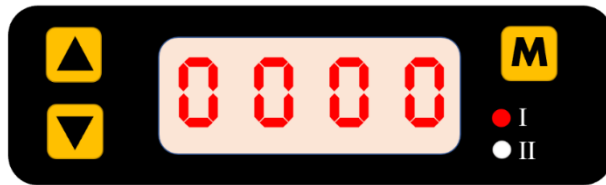
Figure 5.1: MF4700 display and function keys
